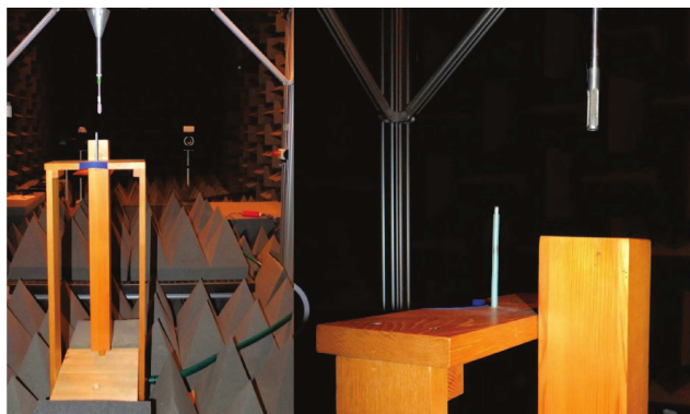
Fig. 6. Sound intensity probe in the lowest position above the upper end of the open pipe.
