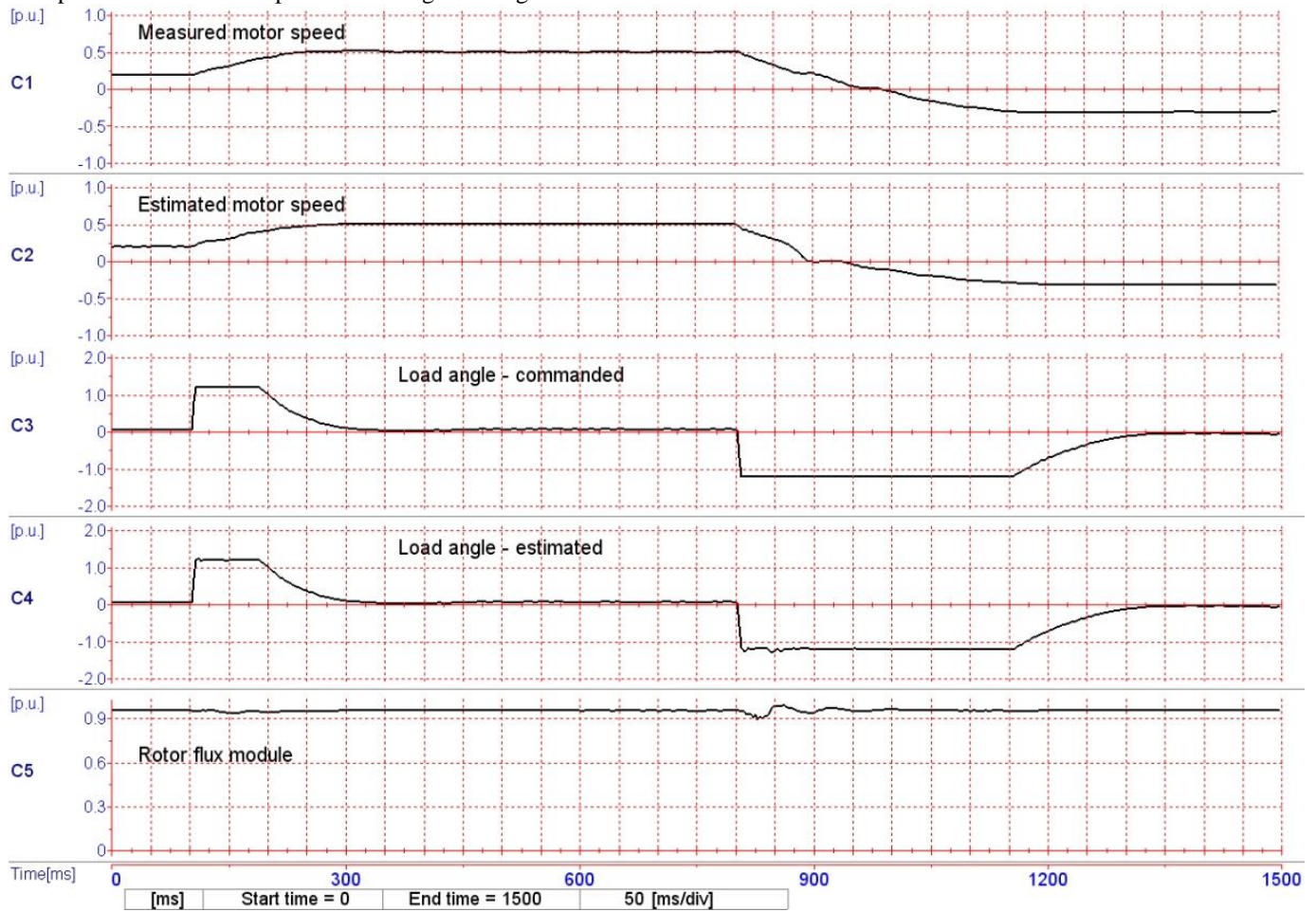
Fig. 16. The speed sensorless induction motor control results in case of the speed variation (Channels: C1- \omega_r , C2- \hat{\omega}_r , C3- \delta^{com} , C3- \hat{\delta} , C5- |\Psi|_r )
