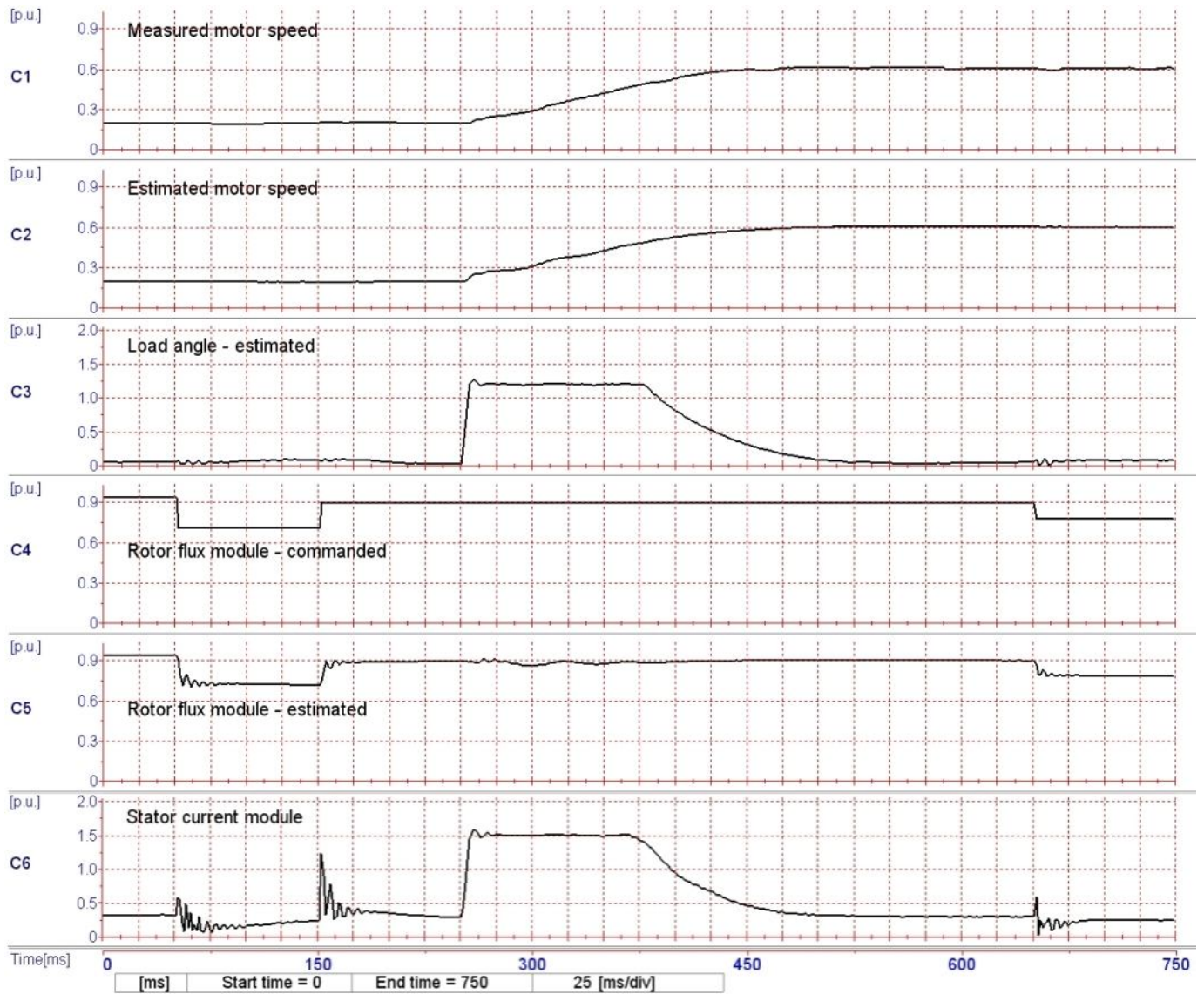
Fig. 17. The speed sensorless induction motor control results in case of the commanded flux and speed variation (Channels: C1- \omega_r , C2- \hat{\omega}_r , C3- \hat{\delta} , C4- \Psi_r^{com} , C5- |\Psi_r| , C6- i_s )
