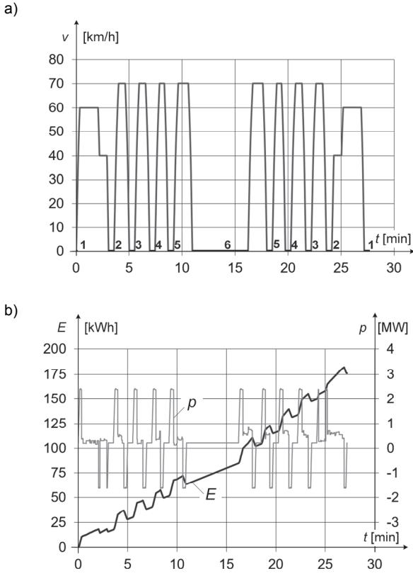
Fig. 4. Conventional EMU run waveforms (Fig. 1): a) train velocity and intermediate stops; b) electrical power and energy usage
