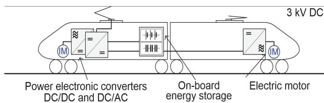
Fig. 2. Examples of EMU drivetrain layout: a) conventional; b) light rail vehicle with on-board storage
