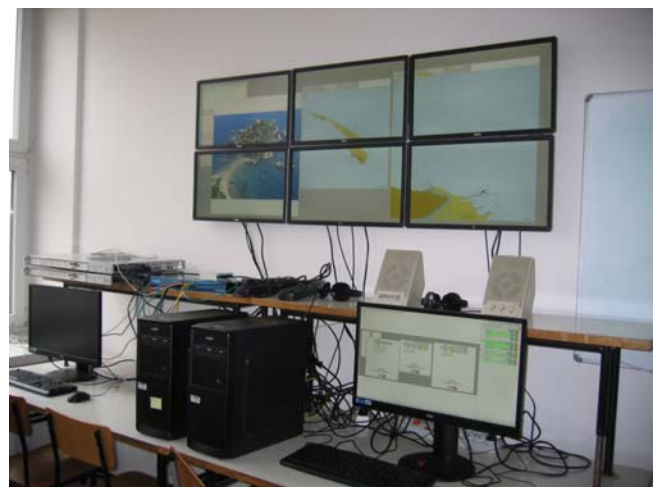
Figure 8. EVP, consisting of multi-display for presentation and standard display for management, during operation.
