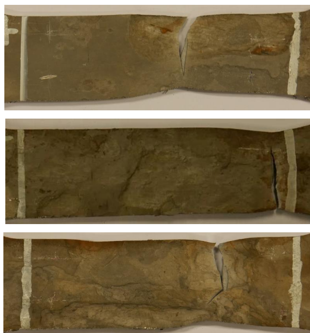
337 Figure 13. The examples of tested specimens with a thickness of 5 mm (top), 6 mm (mid) and 8 mm 338 (bot).
