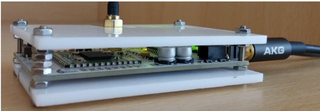
Fig. 5.10. Operating programmable DAB+ receiver.
