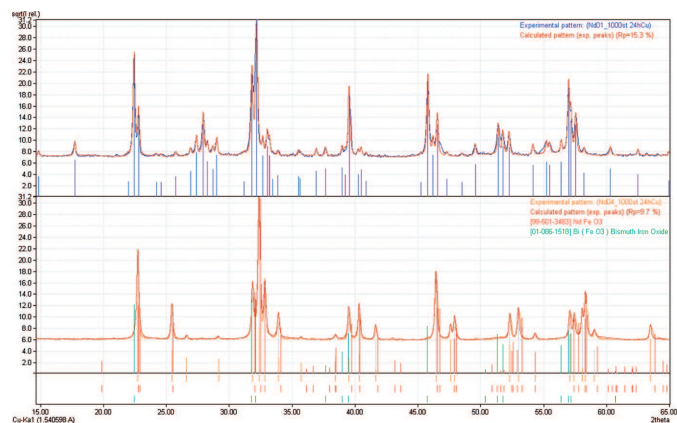
Fig. 7. Results of qualitative X-ray phase analysis of \text{Bi}_{0.6}\text{Nd}_{0.4}\text{FeO}_3 powder
