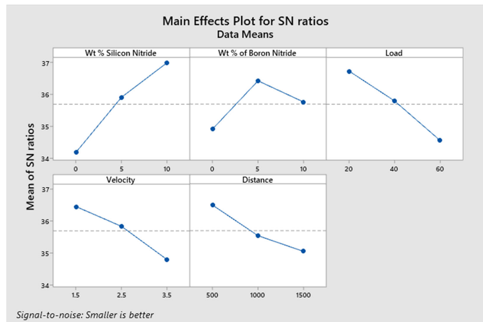
Figure 4. Effect of independent process parameters on the wear rate.
