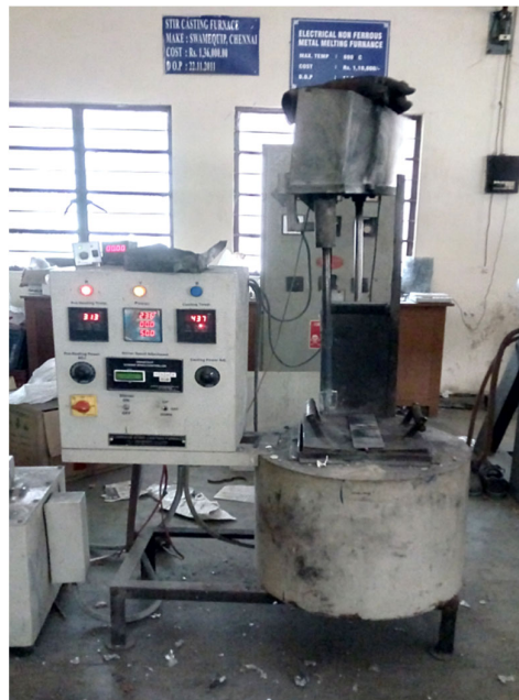
Figure 1. Stir casting setup.
