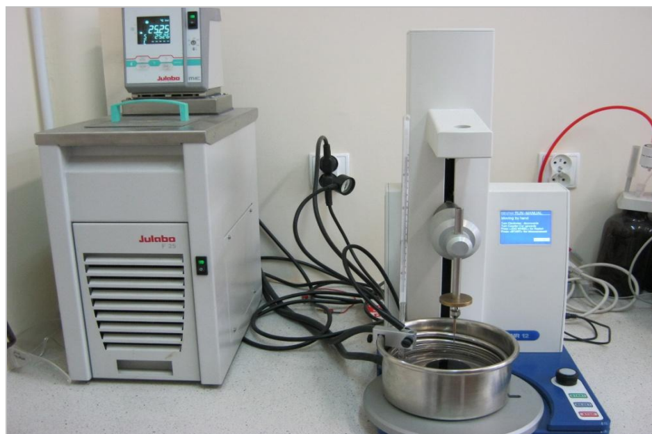
Fig.5.15: Penetration measurement device
