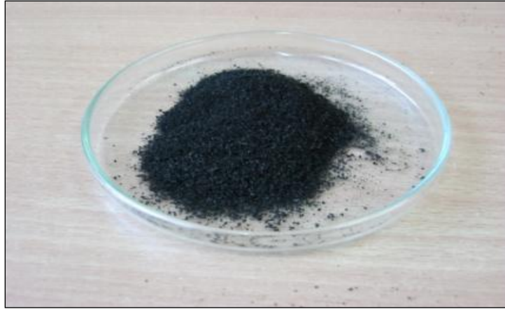
Fig. 1.14: Recycled crumb rubber in particle size less than 0.8 mm [Researcher camera]
