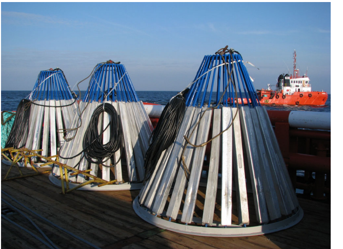
Figure 1 Systems of sacrificial anodes used for the modernization of the platform cathodic protection system
