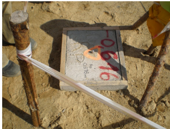
Fig. 10. The central geodetic mark - located in the middle of the stadium plate.
