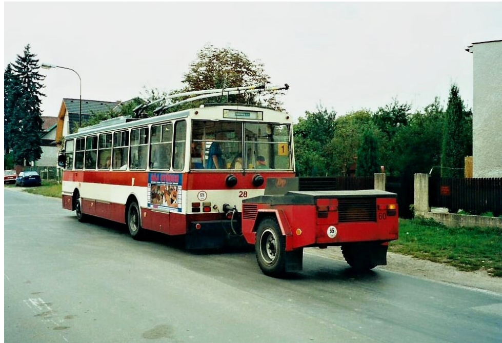
Figure 1. Škoda 14Tr trolleybus with a diesel power generator on the trailer, servicing line no. 1 in Hradec Králové, Czech Republic, from 1994 to 2001 (photo taken by M. Janů).
