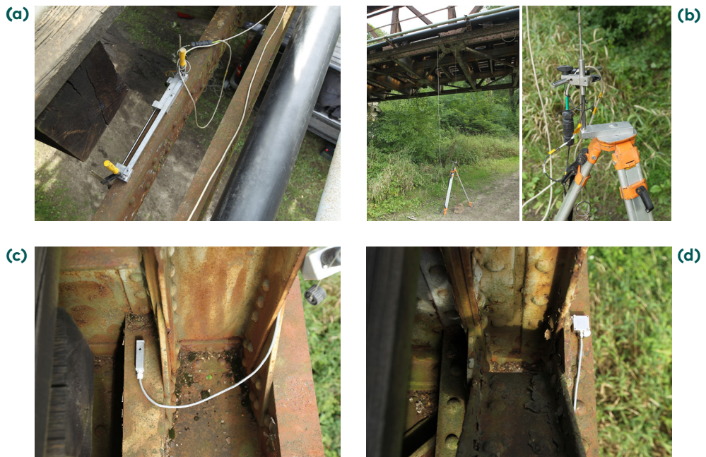
Figure 9. View on chosen measurement points: (a) – Strain measurement point; (b) – Vertical displacement measurement point; (c), (d) – Acceleration measurement points
