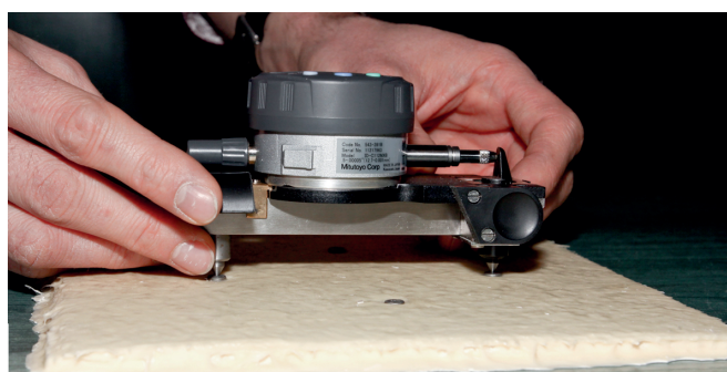
Fig. 5. Extensometer used for length change measurement
