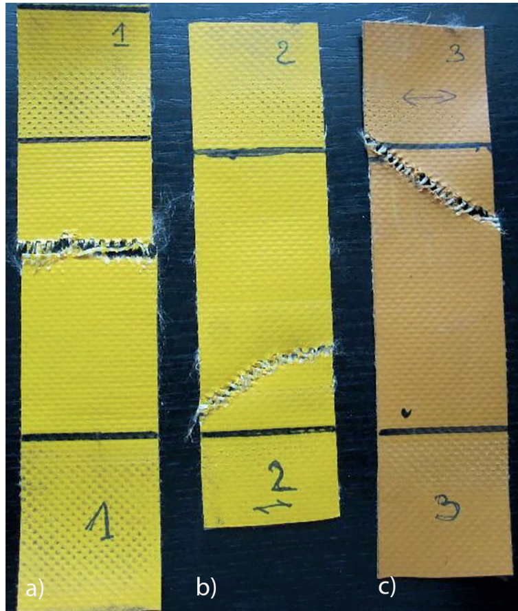
Fig. 4. Specimens after tests (No. 1 and 2 are virgin unused fabric, No. 3 is used fabric).
