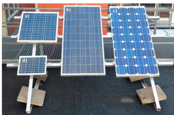
Figure 1. Photovoltaic modules chosen for the annual field study: (a) MWG-30, (b) AP-7105, (c) STP-085, (d) CLC010-12P.
