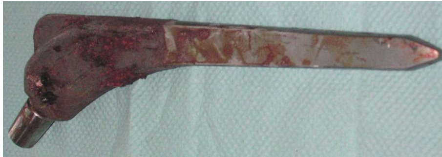
Pic.5. The degraded implants from the second patient
