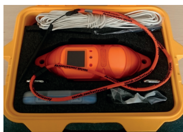
Fig. 11. Sonic sounder for measuring sound speed
