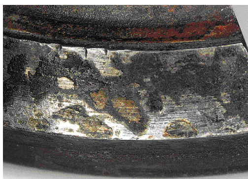
Fig. 3. L12 valve after 3000 hours of operation. Magnification 10x
