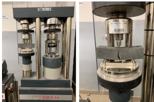
Figure 4. Flexural strength test [Fot.Y.Gu].
