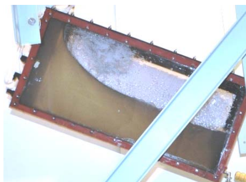
Figure 2. Exemplary shape of a free surface of liquid inside a partly filled model tank (own research) – it may be clearly
