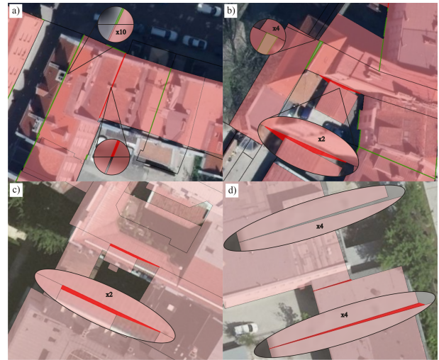
Fig. 6: Four cases considered as the conditional topological errors: a) gap, b) partial c) and d) touching (source: self)
