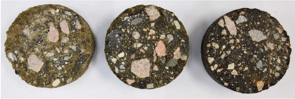
Fig. 2. A typical view of cold in-place recycled mixtures. Samples from left: C2E2, C2E4, C2E6.
