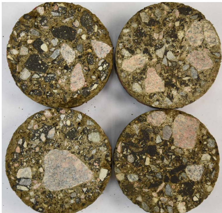
Fig. 3. A display of natural heterogeneity of cold in-place recycled samples. Four samples from one mix type (C6E2).
