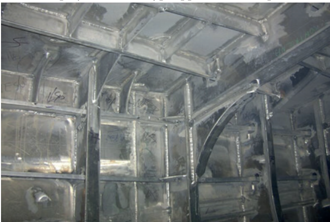
Fig. 1. Typical T-joints in ship structure
