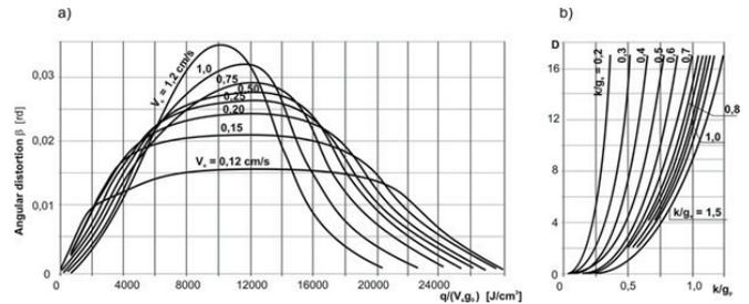
Fig.6. Nomograms: a) for assessing angular distortion  $\beta$  when welding butt welds and T-joints, as functions of welding conditions  $q$ ,  $v_s$ , and calculated plating thickness  $q_0$ , b) for assessing the coefficient  $D$  [14]
