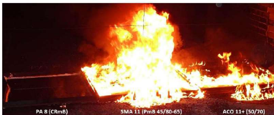
Figure 4 The comparison of the gasoline combustion of the surface of different asphalt mixtures: porous mixture (PA 8), stone mastic asphalt (SMA11, with ~7% of bitumen) and typical asphalt concrete (ACO 11) [23]
