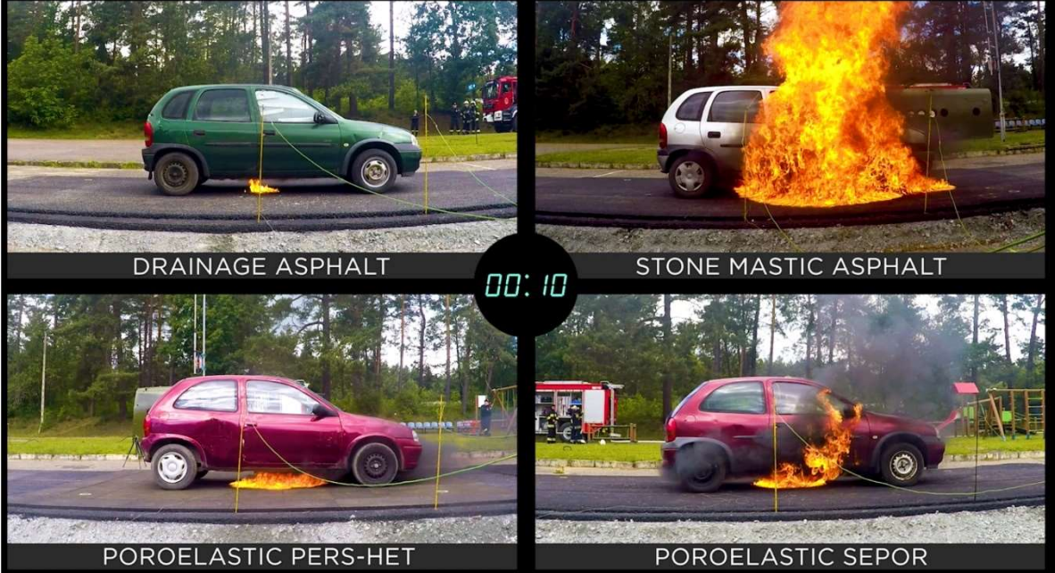
Figure 9. Development of fire 10 s after ignition [27]
