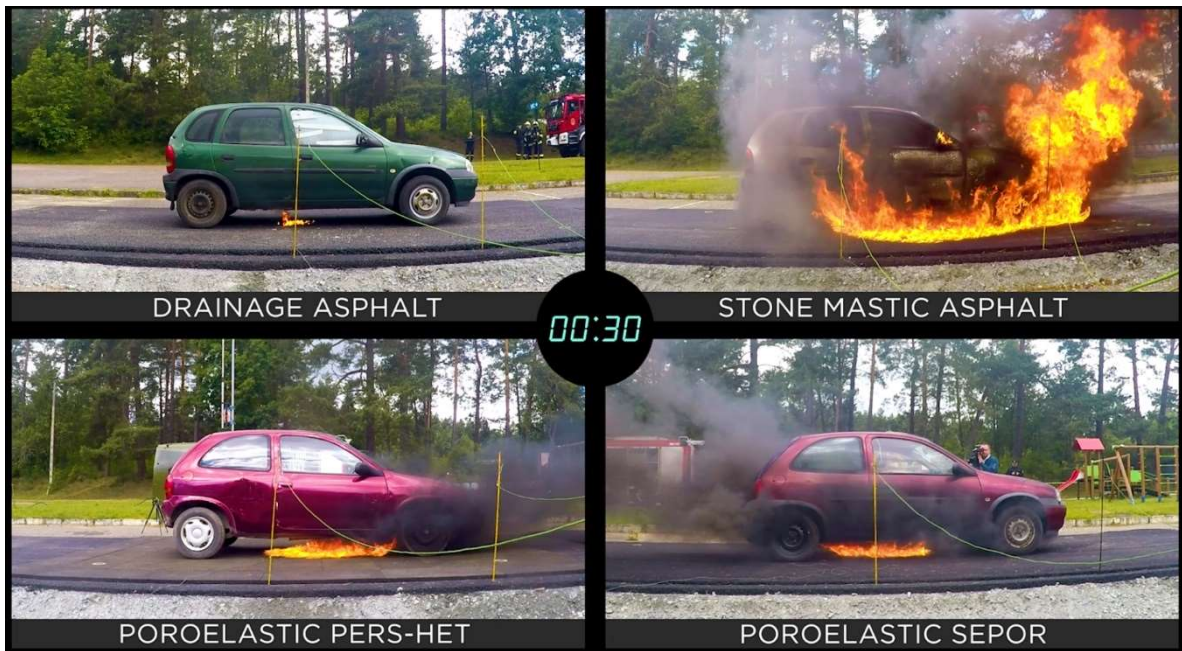
Figure 10. Development of fire 30 s after ignition [27]
