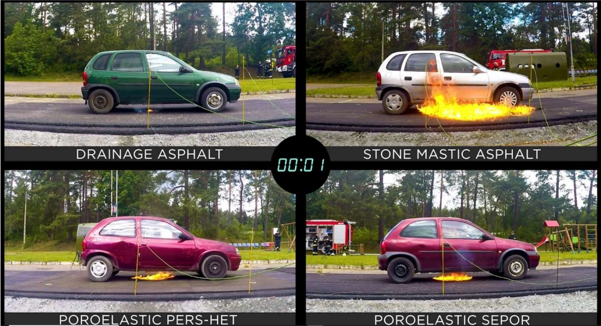
Figure 8. Development of fire 1 s after ignition [27]
