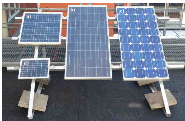
Fig. 2. Photovoltaic modules in natural dust study: a - MWG-30, b - AP-7105, c - STP-085, d - CLC010-12P
