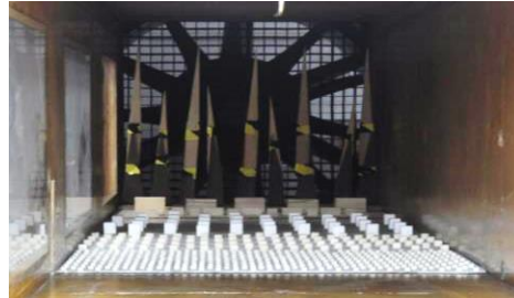
Fig. 2. Elements shaping the profile of velocity
