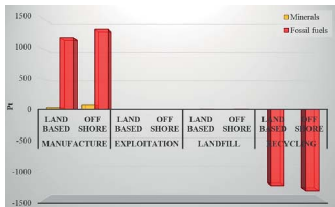
Fig. 12. Results of grouping and weighting of processes leading to depletion of fossil resources, in consecutive stages of material existence cycle of wind power plant blades, taking into account possibility of their post-consumer reuse [own research]
