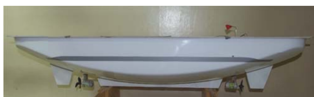
Fig. 7 Side view of the model with appendages
