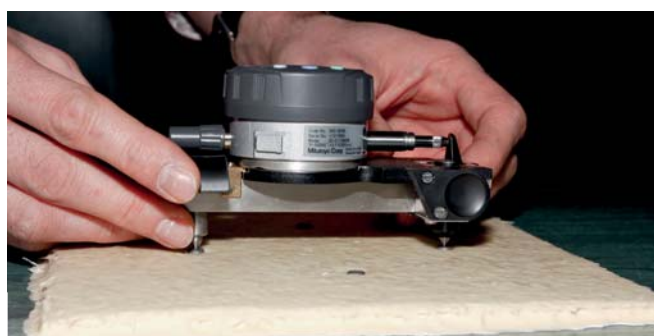
Fig. 5. Extensometer used for length change measurement
