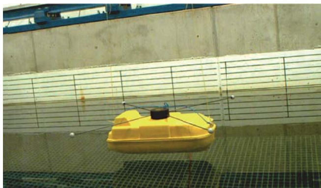
Fig. 1. The lifeboat model suspended on lines with visible QualiSys markers.
