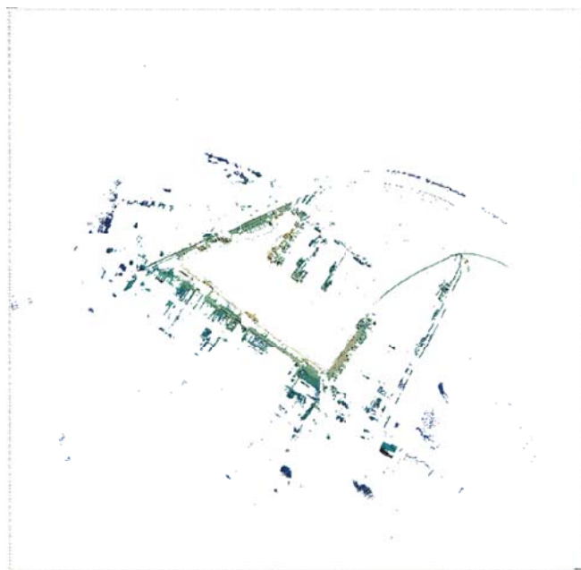
Fig. 12 Cloud of points showing the Port of Władysławowo, originating from scanning from the sea.
