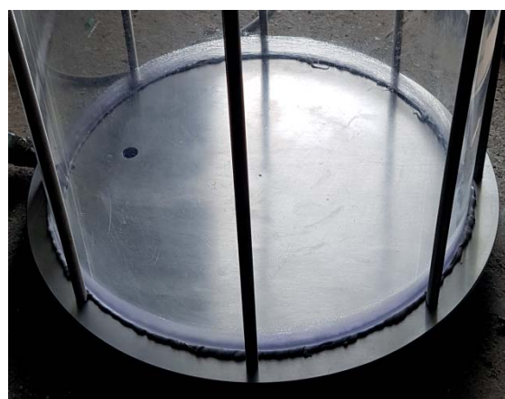
Fig. 8. Sealing of lower tank
