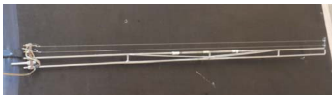
Fig. 3. Resistance probe of the water level manufactured by CTO S.A.
