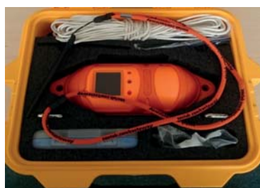
Fig. 11. Sonic sounder for measuring sound speed
