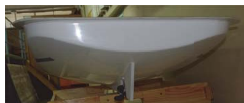
Fig. 8 Front view of the model with appendages
