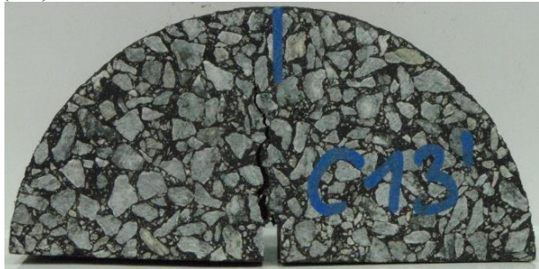
Fig. 3. Stone matrix asphalt SMA 8
