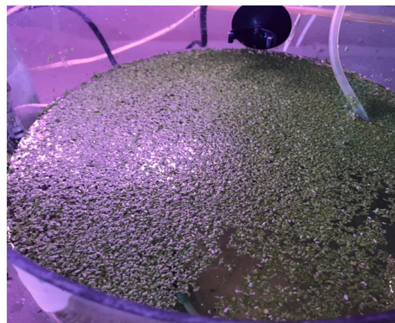
Fig. 1. Phytobioreactor with higher aquatic plants Lemna minor .
