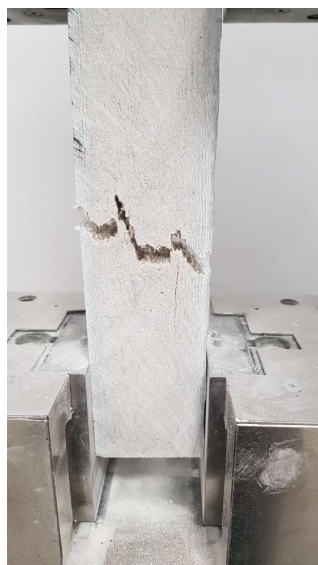
Fig. 7. Axial tensile strength test of GRP pipe
