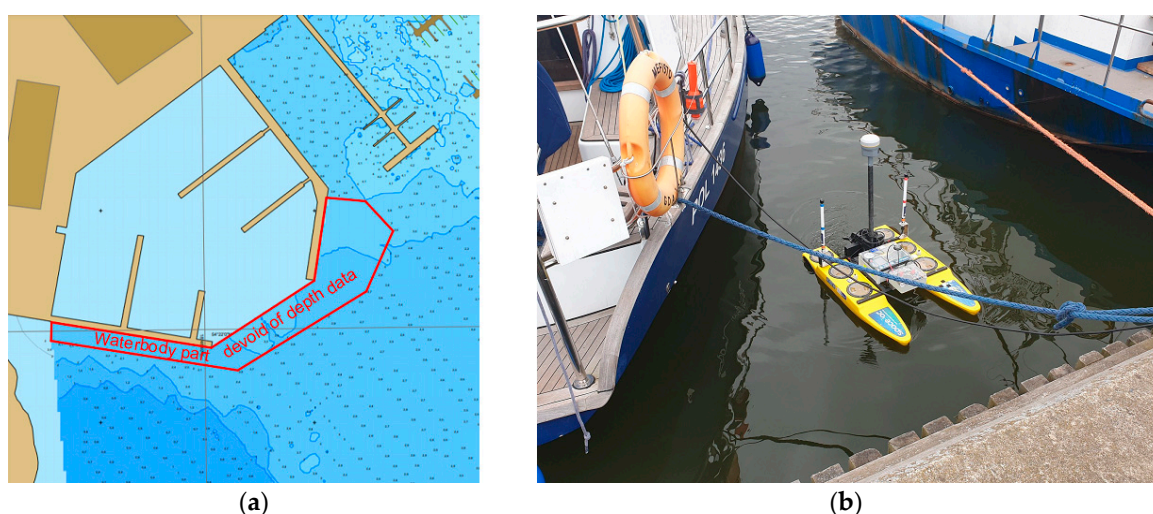
Figure 8. The waterbody in which no surveys were conducted in an automatic mode, due to the yachts moored there (a). A depth measurement between the moored yachts—direct control (b).
