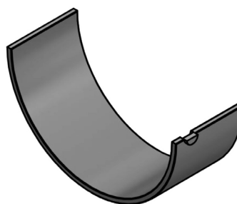
Fig. 2. Axonometric view of the tested bearing. Visible locking lip
