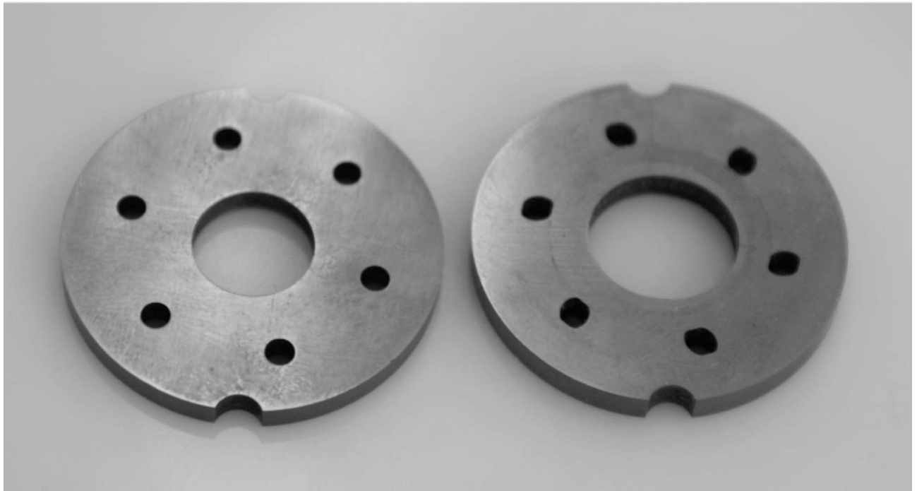
Fig. 27. Commutation plates: high-pressure commutation plate (left) – position 6 in Fig. 25, low-pressure commutation plate (right) – position 7 in Fig. 25.
