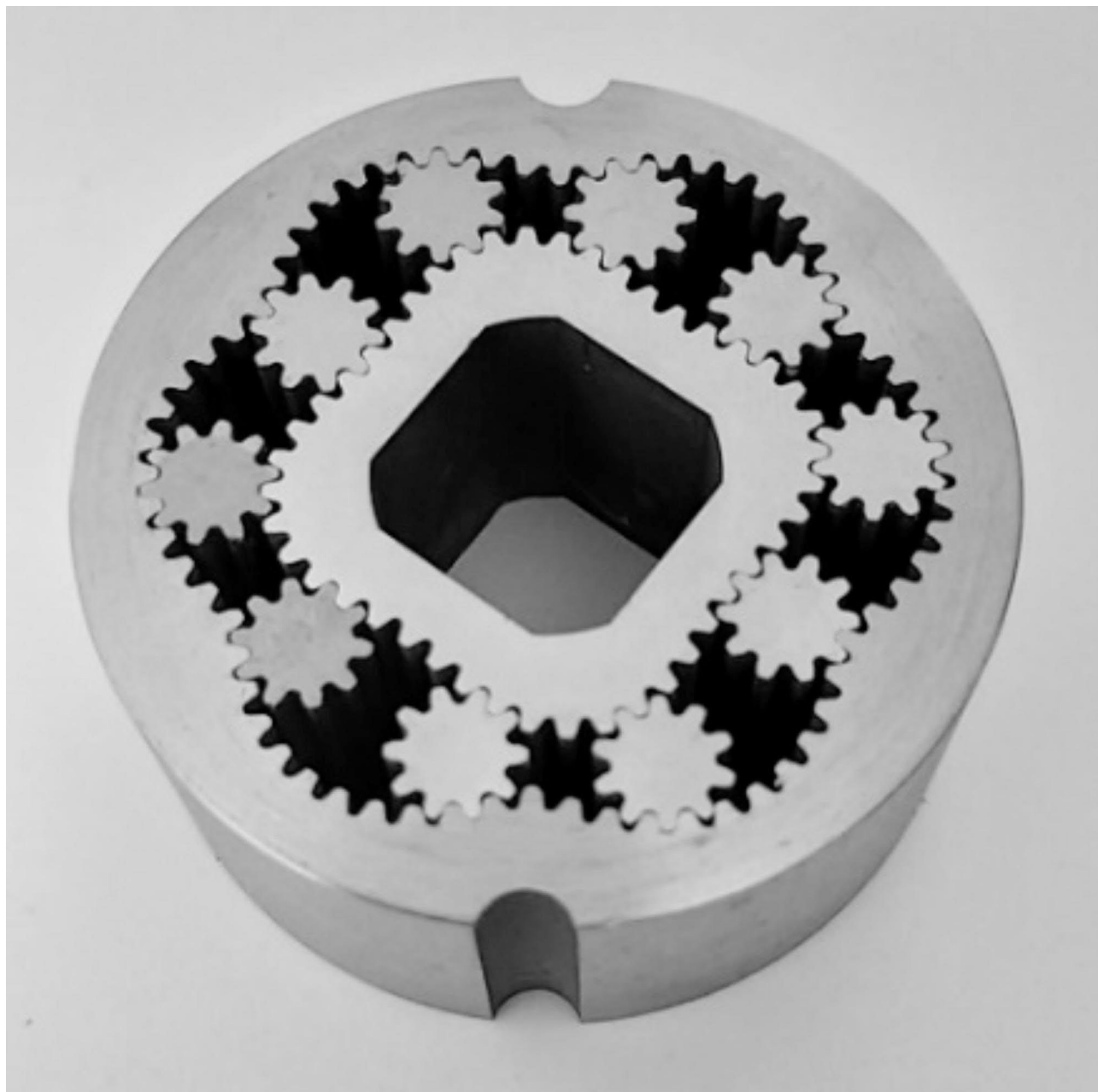
Fig. 26. Satellite mechanism of the tested satellite pump 15,43,44 .
