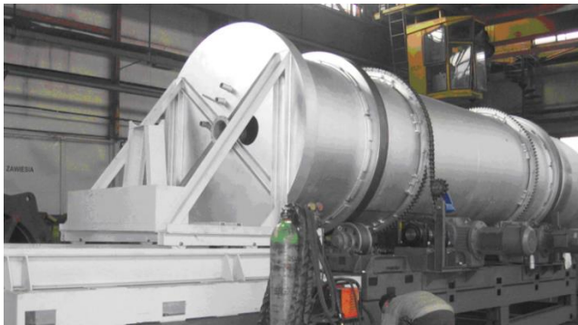
Fig. 3. Detailed view of the rotary pyrolysis chamber.
