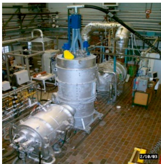
Figure 8. Experimental stand for continuous downdraft gasification.
