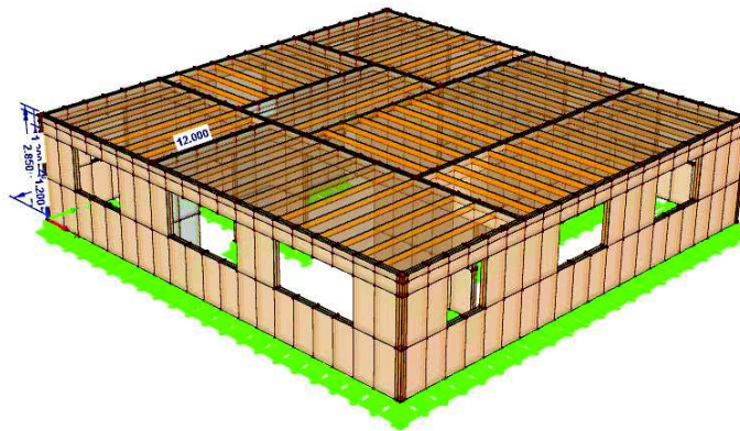
Figure 11. Numerical model of the whole wood-frame house
