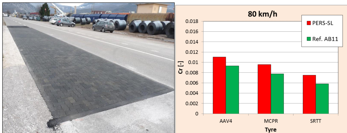
Figure 14. Slovenian test section PERS-SL together with the obtained values of the rolling resistance coefficient on PERS-SL and on the reference AB11 at 80 km/h [3]
