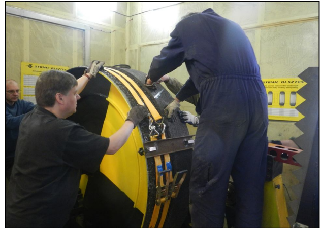
Figure 3. Bonding PERS ribbon to the drum
