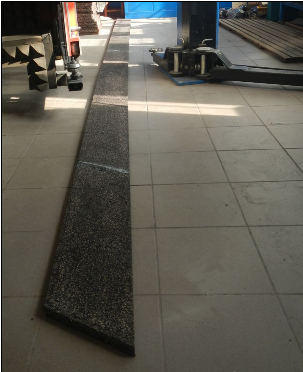
Figure 2. Ribbon formed by joined PERS segments before placing on the drum
