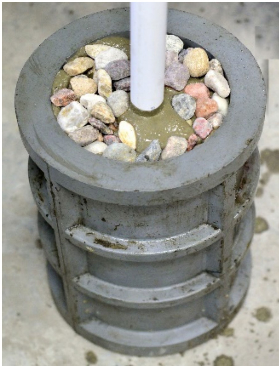
Fig. 3. Injection of grout into the gravels to build a TSC sample.
