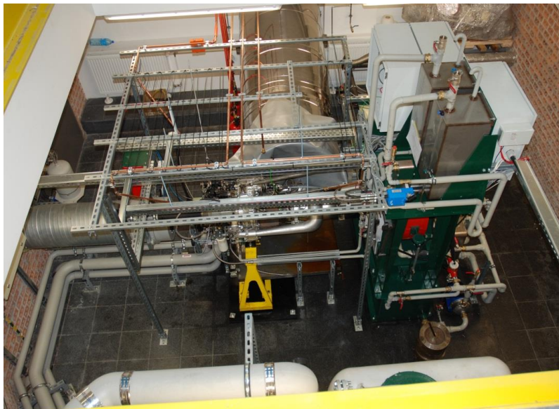
Img 3. Two-shaft gas turbine testing and teaching station
