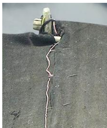
Fig. 126: Method of connection of the two strips of fabric by metal pins
