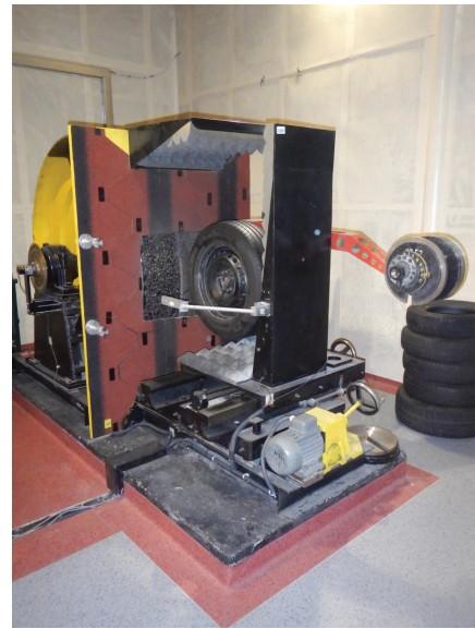
Fig. 4. Roadwheel facility with 1.7m diameter drum at the Technical University of Gdańsk, Poland
