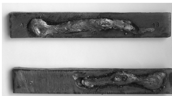
Fig. 11. Specimens with test beads obtained by wet underwater welding conditions with the use of covered electrodes
