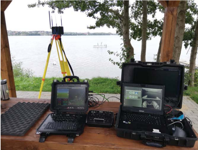
Fig. 19. Fully unmanned vessel system deployed for trials (first plane: shore station, safety pilot, hydrographic console; second plane: shore communication module; third plane: HydroDron unit afloat)
