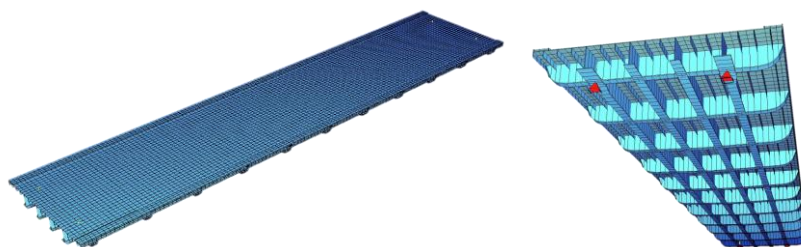
Fig. 2. Discretisation mesh of beam-shell FEM model of footbridge deck [source: own study]
