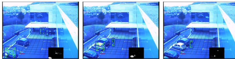
Figure 7: Detection of Cars and People can be used to create interaction rules, such as “Person Out of Car”.
