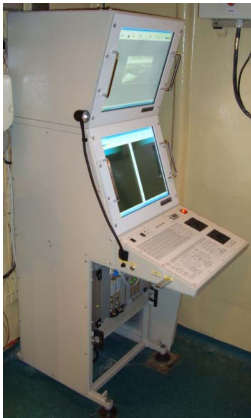
Fig.1. Deck unit – operator console
