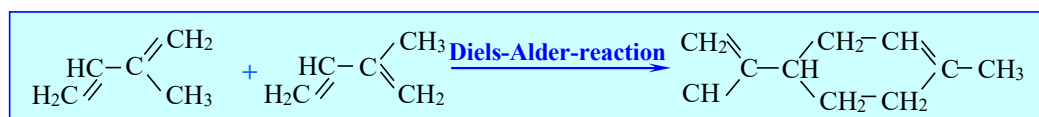
Figure 3. The second pathway of limonene formation from isoprene monomers via the Diels- Alder reaction.
