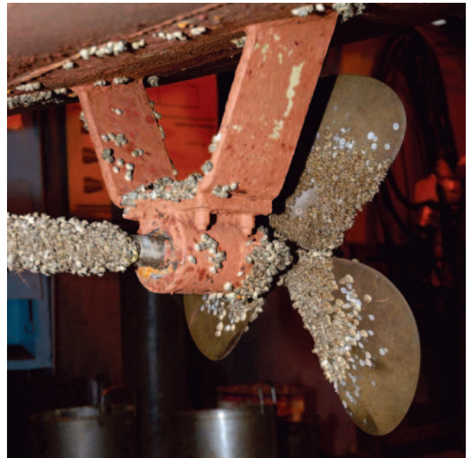
Fig. 2. Cantilever open bearing of yacht's propeller shaft
